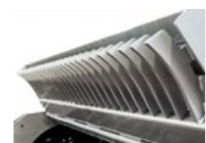
Displacement Chamber this technological solution, which is one of a kind in the industry, allows the ground to be penetrated with the rotor alone
