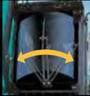
36% larger front wiper wiping area (compared to standard cab)
