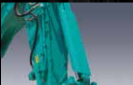
Bucket cylinder guard Prevents damage to the cylinder from falling debris.
