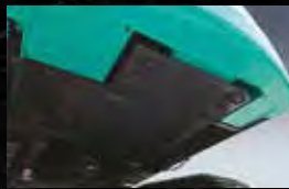
Reinforced upper frame under cover guards 6mm-thick steel plate cover protects devices in the base machine.
