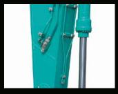
**Piping for Quick Hitch** A quick hitch hydraulic line, which speeds up attachment changes, is available.
