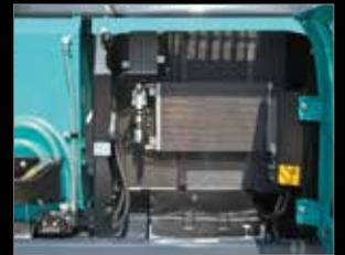
**Left side (radiator and cooling system elements)**
