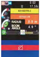
and a warning on the screen if the machine is in a dangerous position. The danger range for tipping differs depending on the upper orientation, due to changes in the level of safety clearance from the swing angle. In longitudinal orientation, a larger maximum working radius can be obtained.
