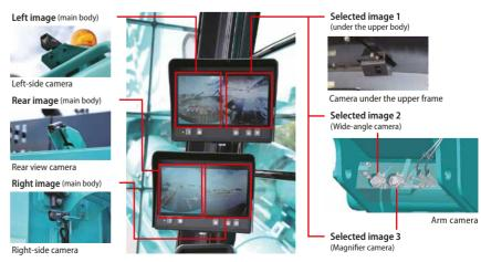
\*The arm camera is only installed on the ultra long attachment.
