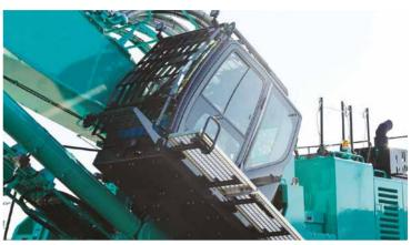
A 30-degree cab tilt angle provides the optimum viewing position when the application requires long periods of working at heights.
